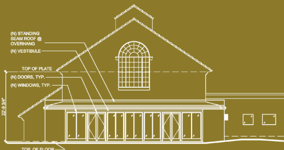
12 EXTERIOR ELEVATION @ SOUTH WALL - MAIN HALL SCALE: 1/8" = 1'-0"
